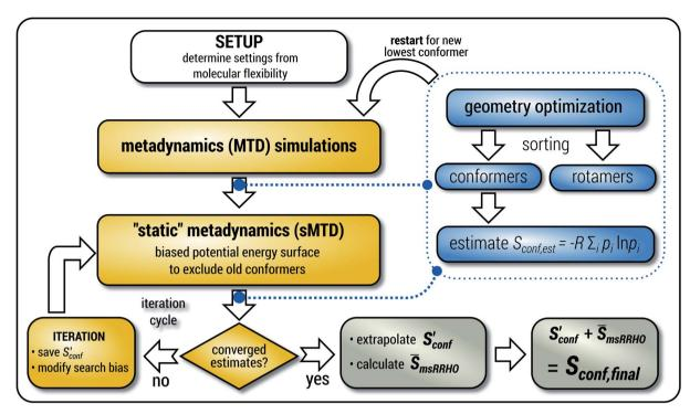
Fig. 1 Schematic representation of the workflow used for the computation of  $S_{conf}$ . See text for details.
