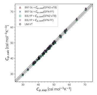
Fig. 6 Parity plots for calculated and experimental heat capacities for a subset of the LBH set. Method combinations of B97-3c and B3LYP-D3/def2-TZVP  $C_{\rm p,msRRHO}$  values with GFN2-xTB and GFN-FF  $C_{\rm p,conf}$  values are shown. UM-VT values were taken from ref. 6.
