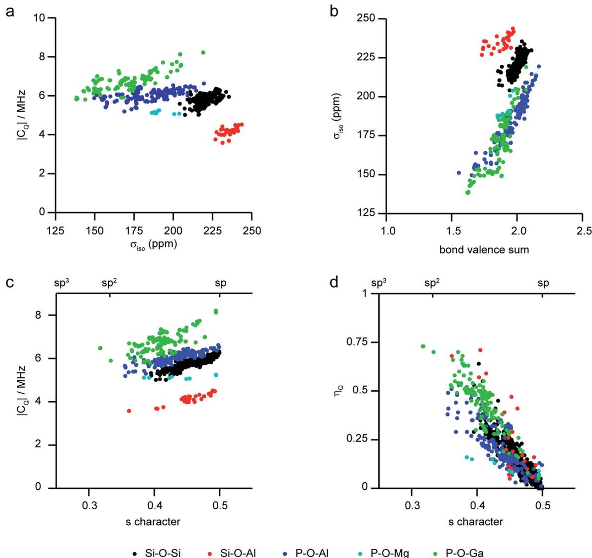
Fig. 4 Plots showing calculated  $^{17}\text{O}$  NMR parameters for a range of model framework solids,<sup>86,91,97–99</sup> coloured by T–O–T' linkage. (a)  $|C_Q|$  against  $\sigma_{\text{iso}}$ , (b)  $\sigma_{\text{iso}}$  against bond valence sum, (c)  $|C_Q|$  and (d)  $\eta_Q$  against the s character of the O bonding.
