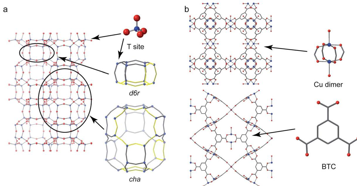
Fig. 1 (a) The structure of CHA zeolite showing the *d6r* and *cha* cage secondary building units (SBUs) with four-, six- and eight-membered rings highlighted. (b) The structure of the Cu-based MOF HKUST-1 (viewed down the (010) and (110) directions) showing the Cu "paddlewheel" dimer and benzene tricarboxylate (BTC) linker building units.
