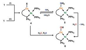
Scheme 3 Synthesis of halo-germylene  ${\rm Ni}^{\rm O}$  complexes 4 and subsequent reactions with NH<sub>3</sub> and H<sub>2</sub>O. (i) 1.1NiX<sub>2</sub>·DME, 2Ph<sub>3</sub>P, 6Zn, THF, 2 h (X = Br); ~24 h (X = Cl); X = Cl and/or Br; (ii) 1Ni(cod)<sub>2</sub>, 2Ph<sub>3</sub>P, toluene, 1 h; X = Cl.
