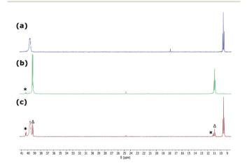
Fig. 3 The  $^{31}$ P{ $^{1}$ H} NMR spectrum of (a) 4b, (b) *in situ* addition of NH<sub>3</sub> to 5b, and (c) 4b regenerated after sonication and degassing the sample used for spectrum (b). \* = small amounts of 6b;  $\Delta$  = small amounts of residual 5b.
