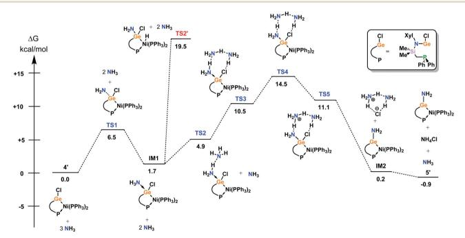
Fig. 5 DFT-derived mechanism for the  $\sigma$ -metathesis of ammonia in 4' leading to 5'.
