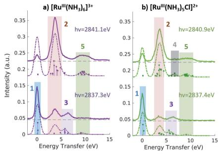
Fig. 5 2p4d RIXS of  $[Ru^{III}(NH_3)_6]^{3+}$  (a) and  $[Ru^{III}(NH_3)_5CI]^{2+}$  (b) measured with incident X-ray energy at the A peak (bottom panels) and B peak (top panels) peak of the respective PFY-XAS spectra and as a function of energy transfer.
