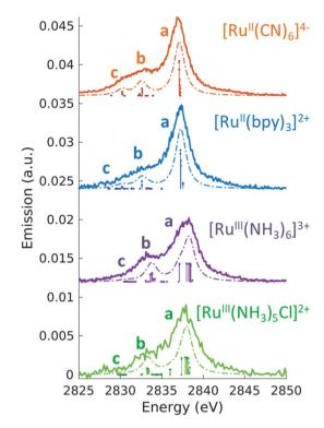
Fig. 3  $4d \rightarrow 2p$  emission (VtC XES, solid line) measured at an incident energy above the ionization threshold of the  $L_3$ -edge (2950 eV). The dashed lines are the TDDFT calculated spectra, obtained by convolving the discrete transitions (vertical sticks) with 1.5 eV (FWHM) Lorentzian function. A global shift of 96.3 eV is applied to the calculated spectra.
