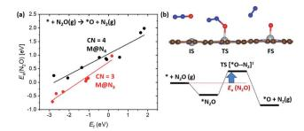
Fig. 5 (a) Shifted linear scaling relationships between  $E_{\rm f}$  and  $E_{\rm a}({\rm N_2O})$  determined by CN. Black and red data points represent M@N $_3$  and M@N $_4$ , respectively. (b) The optimized geometries of the IS, TS and FS for \*O formation when using N $_2$ O and associated energy diagram for  $E_{\rm a}({\rm N_2O})$ .  $E_{\rm a}({\rm N_2O})$  < 0 eV indicates that \*O formation proceeds via exothermic N $_2$ O adsorption and low activation energy.
