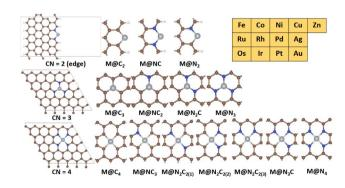
Fig. 2 Calculation models for  $M@N_xC_y$  catalysts. Grey, brown, blue and white balls represent transition metal, carbon, nitrogen and hydrogen atoms, respectively. The 13 late transition metals considered in this study are shown as a table.
