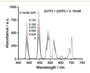
Fig. 12 Ratiometric determination of GTP/GDP ratio using timedelayed luminescence of a mixture of [Tb-2]3+ and [Eu-23]. Reproduced from ref. 61 with permission from the Royal Society of Chemistry, copyright 2013.
