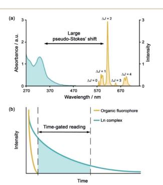
Fig. 1 (a) Representative absorption and emission spectra of Eu(III) complexes highlighting the large pseudo-Stokes'shift; (b) illustration of time-gated detection to eliminate short-lived autofluorescence arising from biomolecules in the sample.
