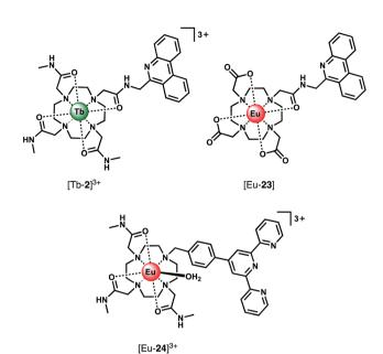
Fig. 11 Eu(III) and Tb(III) complexes capable of selective binding ATP (and GTP) through  $\pi$ - $\pi$  stacking and electrostatic interactions, inducing guenching of luminescence.
