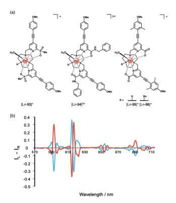
Fig. 20 (a) Family of Eu(III) complexes examined for their ability to signal  $\alpha$ -hydroxy acids (e.g. lactate) by CPL spectroscopy; (b) mirror image CPL spectra of [Eu-56] $^+$  following addition of R-(red) and S-(blue) lactate ( $\lambda_{\text{exc}}=348$  nm, 10  $\mu\text{M}$  complex, 50  $\mu\text{M}$  lactate, 295 K, MeOH). Reproduced from ref.  $^{92}$  with permission from the Royal Society of Chemistry, copyright 2015.
