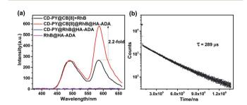
Fig. 4 (a) Gated spectra of CD-PY@CB[8]@RhB (1:0.5:0.02), CD-PY@CB[8]@RhB@HA-ADA (1:0.5:0.02:0.31), CD-PY@RhB@HA-ADA (1:0.02:0.31), and RhB@HA-ADA (0.02:0.31). (b) Decay curves of CD-PY@CB[8]@RhB@HA-ADA (1:0.5:0.02:0.31) at 580 nm ([CD-PY] = 0.5 mM, Ex = 340 nm, Ex. slit = 10, Em. slit = 20, 298 K).
