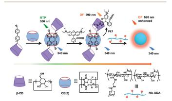
**Scheme 1** Construction of the supramolecular assembly for a purely organic light-harvesting PET system and related molecules.
