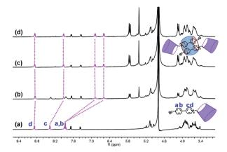
Fig. 1  $\,^{1}$ H NMR titration spectra (400 MHz, D<sub>2</sub>O, 298 K) of CD-PY (1.0 mM) in the presence of (a) 0.00, (b) 0.25, (c) 0.50, and (d) 0.70 equiv. of CB[8].
