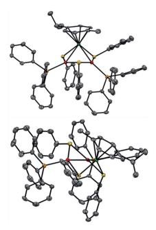
Fig. 4 The crystal structure of Pd<sub>2</sub>Ru complex 1a; ellipsoid drawn at 50% probability, hydrogen atoms and SbF<sub>6</sub><sup>-</sup> anion omitted for clarity; top view (up) and side view (down); Pd (red), Ru (green), S (yellow), P (orange), and C (gray).
