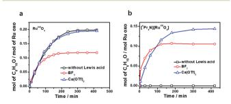
Fig. 1 Time traces for cyclohexane oxidation by (a)  $RuO_4/Lewis$  acid and (b)  $RuO_4^-/Lewis$  acid in  $CH_3CN$ . Conditions:  $RuO_4$  or  $[^{7}Pr_4N]$   $[RuO_4]$  (0.01 M), Lewis acid (0.04 M), cyclohexane (1.0 M) at 23 °C.
