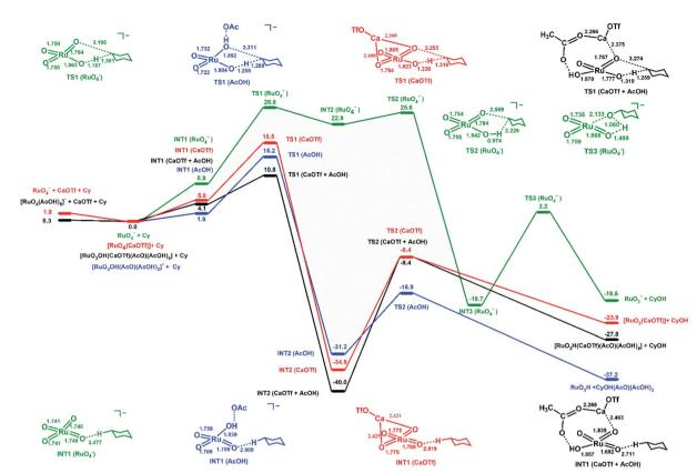
Fig. 7 PESs for cyclohexane oxidation by  $[RuO_4]^-/[RuO_4(AcOH)]^-/[RuO_4(CaOTf)]/[RuO_4(AcOH)(CaOTf)]$  at the B3LYP level using LanL2TZ(f) basis set (Ru) and 6–311++G(d,p) basis set (non-metals). Relative 298 K Gibbs free energies in acetonitrile are given in kcal mol<sup>-1</sup>. Not all acetic acid molecules are shown for simplicity.
