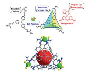
Fig. 24 Supramolecular cages self-assemble when a ligand and  $\mathrm{Co}^{2+}$  ions are combined in a 1:1 stoichiometry. The cage encapsulates an organic fluorescein photosensitizer in a following step. The assembly is an efficient light drive proton reduction catalyst. Used with permission from ref. 112.
