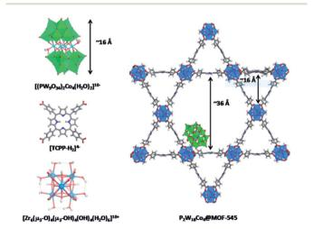
Fig. 18 The components (left) are the catalytic POM (top) light-harvesting porphyrin strut (middle) and structural Zr-cluster (bottom) that lead to a supramolecular artificial photosynthetic assembly (right). Used with permission from ref. 99.
