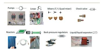
Fig. 2 Flow equipment and representation.
