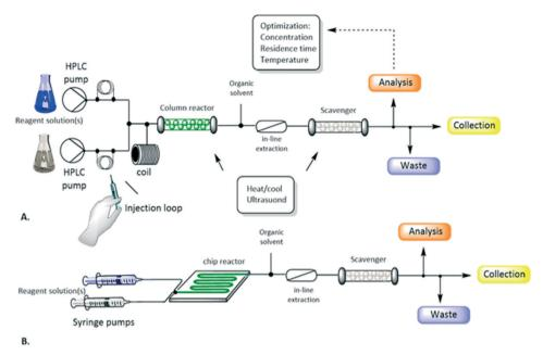
Fig. 1 Schematic representation of a flow reactor configuration involving mesoreactors (A) or microreactors (B). Figure adapted from Tamborini et al.<sup>59</sup>
