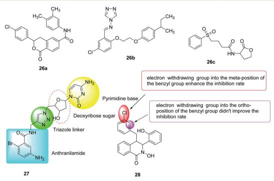
Fig. 18 Structure of compounds 26a-c, 27 and 28.
