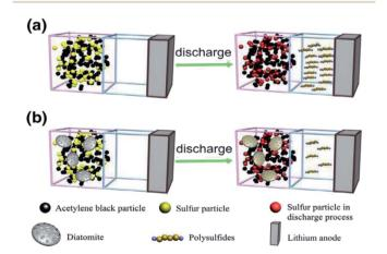
Polysulfide suppression behaviour schematically illustrated for (a) sulfur electrode without DE (b) sulfur electrode with DE.83
