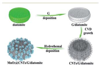
Fig. 8 Illustration of the MnO2@CNTs/G/diatomite composite fabrication. 105
