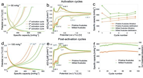
Fig. 5 The electrochemical performance of the milled and pristine DE-based negative electrodes: (a and d) voltage profile curves, (b and e) differential capacity plots, (c and f) specific capacity against cycle number for activation (a–c) and post-activation (d–f) curves (green points: milled DE) and (orange points: pristine DE).<sup>63</sup>
