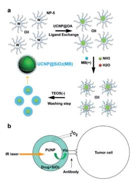
Fig. 3 (a) The formation mechanism of NaYF4:Er/Yb/Gd@SiO $_2$  (MB) in the water-in-oil reverse microemulsion system.<sup>59</sup> (b) Schematic of the design of the versatile photosensitizer based on photon upconverting nanoparticles.58
