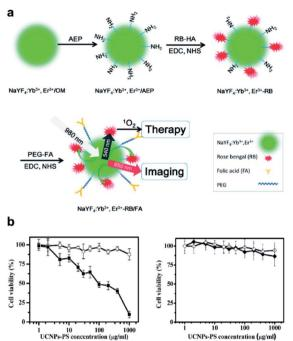
Fig. 7 (a) Schematic of covalent conjugation of NaYF<sub>4</sub>:Yb<sup>3+</sup>, Er<sup>3+</sup> UCNPs, photosensitizer RB, and target molecule FA. (b) Viability of JAR cells (left) and NIH 3T3 fibroblasts (right) treated with UCNPs-PS of different concentrations with (solid) or without (open) 980 nm exposure. $^{70}$
