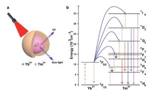
Fig. 1 (a) Illustration of the energy transfer mechanism of the coreshell NaGdF4:Yb/Tm@NaGdF4 UCNPs. The energy transfer occurs through the Yb  $\rightarrow$  Tm pathway upon 980 nm excitation. (b) Energy level diagrams of the Yb<sup>3+</sup> and Tm<sup>3+</sup> ions and the energy transfer mechanism of the UCNPs in the energy level.
