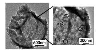
Fig. 7 TEM micrographs of Pd/[BMIM][PF $_6$ ] in SiO $_2$ , with black circles highlighting Pd nanoparticle formation within the capsules. [Reprinted with permission from ref. 32. Copyright (2014) American Chemical Society].
