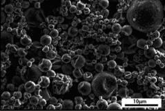
Fig. 4 SEM micrographs of [BMIM][PF<sub>6</sub>] in polyurea capsules prepared *via* emulsion polymerization in water (top) and in oil (bottom). [Reprinted from *React. Funct. Polym.*, Weiss, E.; Gertopski, D.; Gupta, M. K.; Abu-Reziq, R. Encapsulation of Ionic Liquid BMIm[PF<sub>6</sub>] within Polyurea Microspheres. 2015, 96, 32–38, with permission from Elsevier]. 42
