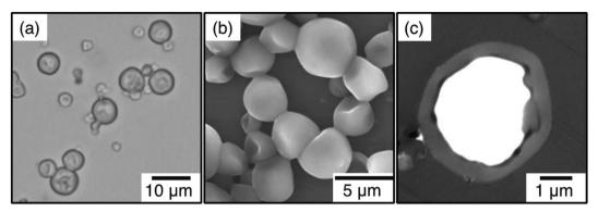
Fig. 3 Optical micrograph (a), SEM (b), and TEM micrograph of ultrathin cross-section (c) of poly(triethylene glycol dimethacrylate/n-butyl methacrylate)/[HMIM][TFSI] (P(TEGDM-BMA)/P(BMA)/[HMIM][TFSI]) composite particles prepared by microemulsion polymerization. [Reprinted with permission from ref. 41. Copyright (2013) Springer].
