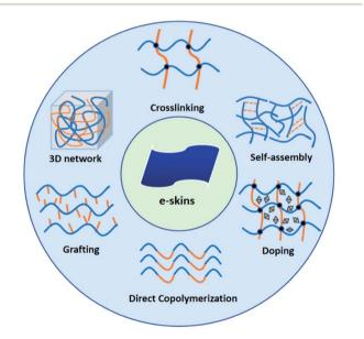
Fig. 1 Illustration of structural designs and methodologies to fabricate conductive hydrogels in the application of e-skins.
