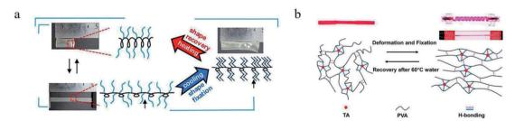
Fig. 3 (a) The shape memory process and mechanism of a SMP with spring-like main chains and comb teeth-like side chains.<sup>35</sup> Copyright 2019. Reproduced with permission from American Chemical Society. (b) Shape memory mechanism of the PVA-TA Hydrogel.<sup>46</sup> Copyright 2016. Reproduced with permission from American Chemical Society.
