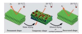
Fig. 4 A schematic illustration of the shape memory process of a SMP accompanied by reconfiguration of photonic crystals.<sup>57</sup> Copyright 2015. Reproduced with permission from Springer Nature.
