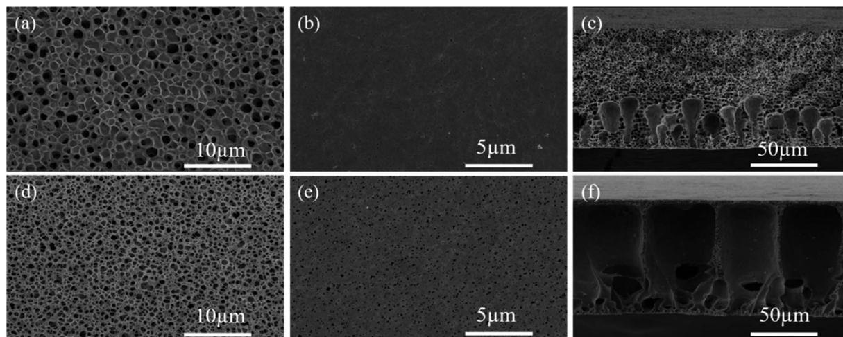
Fig. 1 SEM images of (a) bottom surface, (b) top surface and (c) cross section of PVDF-HFP membrane. SEM images of (d) bottom surface, (e) top surface and (f) cross section of PVDF-HFP-PEO-SiO<sub>2</sub> membrane.
