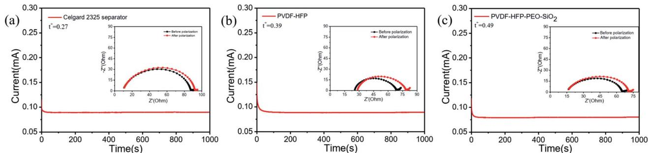
Fig. 5 Chronoamperometry curves of (a) Celgard 2325 separator, (b) PVDF-HFP, (c) PVDF-HFP-PEO-SiO<sub>2</sub> in the symmetrical Li/GPE/Li cells. AC impedances before and after polarization are shown in the inset.
