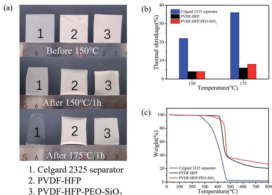
Fig. 2 (a) Photographs of the Celgard 2325 separator and PVDF-HFP-based membranes before and after being exposed to 150 °C and 175 °C for 1 h. (b) Thermal shrinkage of membranes after heat-treatment. (c) TG curves for various membranes.
