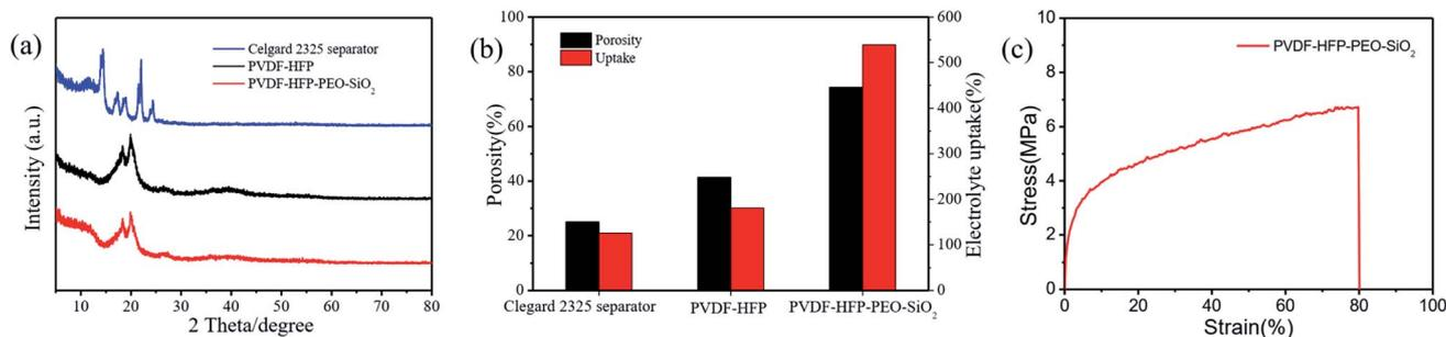
Fig. 3 (a) XRD patterns, (b) porosity and electrolyte uptake of the Celgard 2325 separator, pure PVDF-HFP and PVDF-HFP-PEO-SiO<sub>2</sub>, (c) stress-strain curve of the PVDF-HFP-PEO-SiO<sub>2</sub> GPE.
