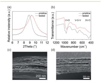
Fig. 4 Investigation of the pristine and electrochemical tested  $V_2O_5$  cathode by (a) XRD and (b) FTIR. SEM cross-section images of the (c) pristine and (d) tested cathode, showing the preservation of the structural integrity of the  $V_2O_5$  cathode upon electrochemical cycling.
