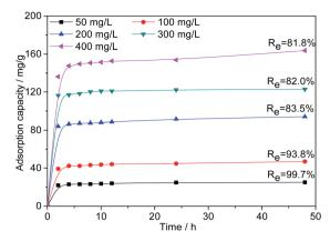
Fig. 9 Effects of contact time and initial concentration on the adsorption capacity of Cr(vi) on AC-3.0-700.
