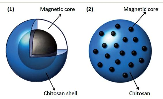
Fig. 4 Two types of coating magnetic core in chitosan, this figure has been adapted from ref. 108 with permission from Elsevier B.V., copyright 2013.
