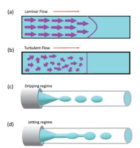
Fig. 6 (a) Laminar flow, (b) turbulent flow, (c) dripping regime, and (d) Jetting regime.
