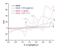
Fig. 1 Cyclic voltammograms recorded on a glassy carbon electrode at 100 mV s $^{-1}$ : (a) blank solution, 0.1 M  $n\text{-Bu}_4\text{NBr}$  in DMA; (b) solution (a) with 7.5 mM NiCl $_2$ ·glyme added; (c) solution (a) with 7.5 mM 2,9-dimethyl-1,10-phenanthroline added; and (d) solution (a) with 7.5 mM NiCl $_2$ ·glyme and 2,9-dimethyl-1,10-phenanthroline (Ni/L = 1/1) added.
