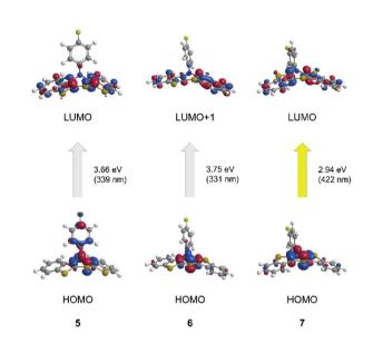
Fig. 10 TDDFT calculated frontier molecular orbital (FMO) transitions of the longest wavelength absorptions of the neutral compounds 5, 6, and 7 (B3LYP/6-311++G\*\*, IEFPCM CH<sub>2</sub>Cl<sub>2</sub>, isosurface value 0.05 a.u.).
