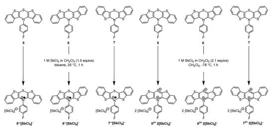
Scheme 3 Controlled preparation of oxidized BBTT-compounds 5<sup>++</sup>, 6<sup>++</sup>, 7<sup>++</sup>, and 5<sup>2+</sup>, 6<sup>2+</sup>, 7<sup>2+</sup> as hexachloroantimonates using antimony pentachloride as an oxidant.
