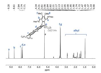
Fig. 3  $\,^{1}$ H NMR spectrum (700 MHz, CD<sub>2</sub>Cl<sub>2</sub>) of cage (R,R)-9. # residual CH<sub>2</sub>Cl<sub>2</sub>.
