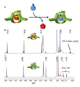
Fig. 6 (a) Exchange of host molecules from THF@(R,R)-9 to toluene-d8@(R,R)-9. (b) <sup>1</sup>H NMR spectrum (700 MHz) of freshly prepared THF@(R,R)-9 in toluene-d8. (c) same sample after exchange of THF guest by toluene-d8. Note, that in the upper spectrum some toluene-d8@(R,R)-9 has formed.
