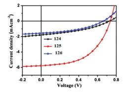
Fig. 22 Current-voltage characteristics of optimized photovoltaic cells based on 124: PC<sub>61</sub>BM, 125: PC<sub>61</sub>BM and 126: PC<sub>61</sub>BM under illumination of AM 1.5, 100 mW cm<sup>-2</sup> white light. Reproduced with permission of Elsevier.74
