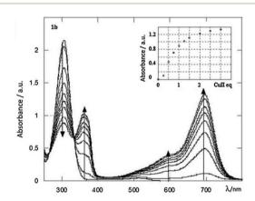
Fig. 5 UV-vis absorption spectra of a  $5 \times 10^{-6}$  mol dm<sup>-3</sup> solution of 58b upon gradual addition of copper perchlorate in acetonitrile. Inset, increase of the 696 nm peak with the number of Cu(II) equivalents. Reproduced with permission of Elsevier. 46
