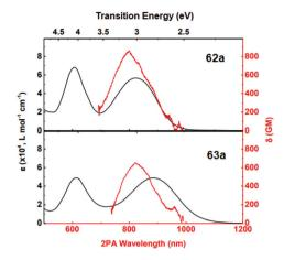
Fig. 8 Linear (black curves, scale upwards) and two-photon (red curves, scale downwards) absorption spectra of 62a, 63a in DCM. Adapted from ref. 47 with permission from The Royal Society of Chemistry.
