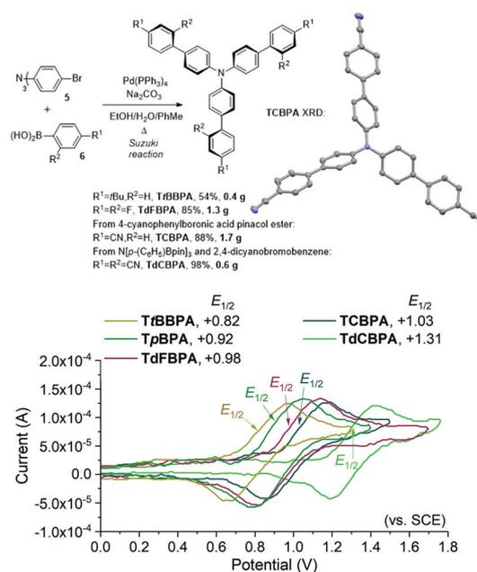
Fig. 4 Second Generation of TPA e-PRCats, and the XRD structure of **TCBPA** (top). Thermal ellipsoids are set at the 50% probability level. H atoms omitted for clarity. C atoms (grey), N atoms (blue). Cyclic voltammetry (bottom).
