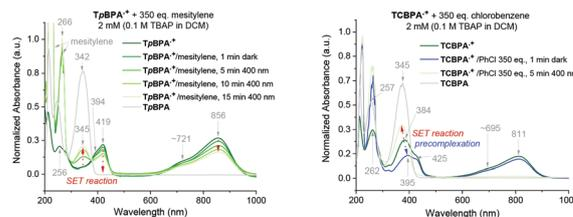
**Fig. 9** UV-vis spectra of **TpBPA<sup>+</sup>** (top) and **TCBPA<sup>+</sup>** (bottom) in the presence of mesitylene and PhCl, respectively and after irradiation at 395 nm.
