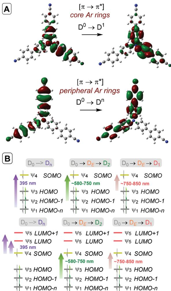
**Fig. 15** (A) Natural Transition Orbitals (NTOs) depicting photoexcitation of  $\text{TCBPA}^{+\bullet}$  to  $D_1$  or  $D_n$ . (B) TD-DFT predicted orbital transitions of  $\text{TpBPA}^{+\bullet}$  (top) and  $\text{TCBPA}^{+\bullet}$  (bottom). Wavelengths are derived from optical transitions.
