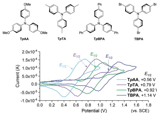
Fig. 2 First generation TPA e-PRCats (top). Cyclic voltammograms (bottom).
