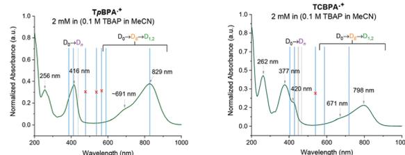
Fig. 14 Computed (CAM-B3LYP/6-31G(d,p), CPCM = MeCN, blue lines) vs. experimental UV-vis spectra of TpBPA<sup>+</sup> and TCBPA<sup>+</sup> in MeCN containing 0.1 M <sup>n</sup>Bu<sub>4</sub>N<sup>+</sup>PF<sub>6</sub><sup>-</sup>. Negligible TD-DFT excitations (coefficient  $f < 0.0020$ ) in grey. Assignments based on the optical transitions.
