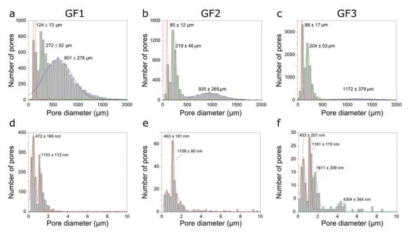
Pore width distributions of samples GF1, GF2 and GF3 obtained using micro-CT (a-c), and nano-CT (d-f)
