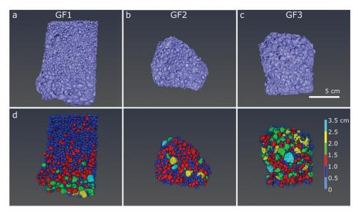
Fig. 4 Reconstructed 3D micro-CT images of samples (a) GF1, (b) GF2 and (c) GF3, and segmented pores with color-coded diameter shown below, in (d-f). Scale bar: 5 μm.
