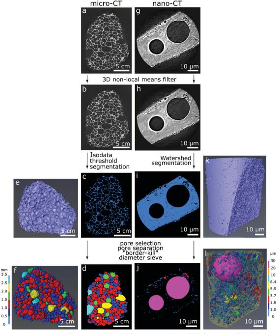
Fig. 1 Image processing workflow for the CT datasets using sample GF2 as example. Left: Micro-CT (a-f); right: nano-CT (g-I). The original grey scale reconstructed slices (a and g) were filtered (3D non-local means), resulting in (b and h). After segmentation (c and i), volumetric representations were obtained (e and k). After processing, the pore visualization is possible in two- (d and j) and in three-dimensions (f and l) for micro-CT and nano-CT.
