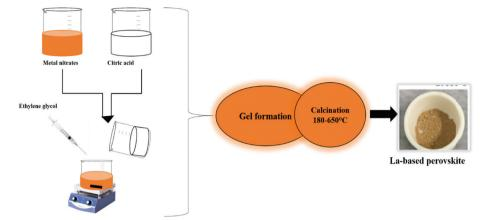
Scheme 2 Schematic diagram illustrating sol-gel synthesis of La-based perovskites.
