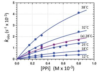
Fig. 5 Individual L.S. fits of  $k_{obs}$  vs. [PPi]<sub>tot</sub> (eqn (1)) at different temperatures and pH 7.35 ([Tris buffer] = 10 mM). (a) The purple line indicates the profile obtained from the F.I. vs. time traces at 28 °C. A global fit was additionally performed to determine the activation parameters (sections \$1.1, \$4, and Fig. \$6†).
