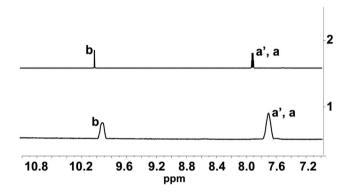
Fig. 2 Line 1: <sup>1</sup>H NMR spectra of 1-OH<sub>2</sub>\* (2 mM) in the presence of PPi (10 equiv.: 20 mM: incubation time: 30 min) at pD 7.35 (D<sub>2</sub>O. [Tris buffer] = 10 mM). Line 2: <sup>1</sup>H NMR spectra of pure signaling aldehyde 4 in D<sub>2</sub>O. Characteristic protons are indicated in Fig. 1A. \* The <sup>1</sup>H NMR spectrum of 1-OH2 did not show any signal in this region due to the paramagnetism of the probe.
