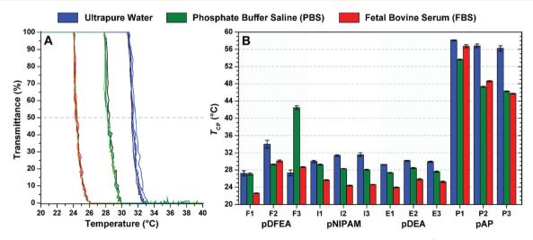
Fig. 3 (A) Comparison of 6 turbidimetric measurements of I2 (pNIPAM) in water, PBS and FBS ( $c = 10.0 \text{ mg mL}^{-1}$ ); (B)  $T_{CP}$  of all polymers in water, PBS and FBS ( $c = 10.0 \text{ mg mL}^{-1}$ ) expressed as a mean of 6 measurements  $\pm$  standard deviation. The results indicate a shift in  $T_{CP}$ .
