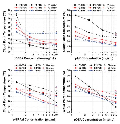
Fig. 4 Plot of  $T_{CPS}$  of the polymers pDFEA (top-left), pAP (top-right), pNIPAM (bottom-left) and pDEA (bottom-right) in FBS and PBS as a function of polymer concentrations. All  $T_{CPS}$  are expressed as the mean of 6 measurement cycles  $\pm$  standard deviation. Asterisks (\*) indicate potential outliers.
