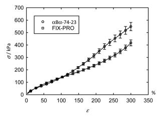
Fig. 4 Average tensile performance for  $\alpha B\alpha$ -74-23 and FIX-PRO® are given as squares and circles respectively, showing similar tensile performance up to 120% strain. Error bars denoting  $\pm$ one standard error at symbols are given for clarity, with lines through data representing the full curve in each case.
