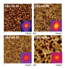
Fig. 3 AFM images for each of the synthesised  $\alpha B\alpha$  triblock copolymers (height images), with FFTs shown as an insert.  $1 \times 1 \mu m$  area shown. Lighter areas correspond to the PaPMA domains and darker regions correspond to the PBuA domains.
