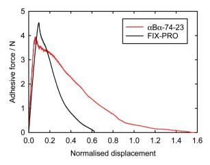
Fig. 6 Representative probe adhesion results for single specimens of  $\alpha B\alpha$ -74-23 and FIX-PRO® to full detachment.  $W=69.3~\rm kJ~m^{-3}$  for  $\alpha B\alpha$ -74-23, and 39.5 kJ m<sup>-3</sup> for FIX-PRO® were determined from the areas under the curves.
