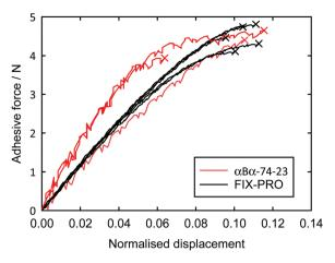
Fig. 5 Adhesive probe tack force as a function of displacement normalised by specimen thickness, for 3 specimens of  $\alpha B\alpha$ -74-23 and for 5 specimens of FIX-PRO®. Crosses indicate failure properties for both materials.
