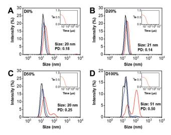
Fig. 2 Size distributions of (A) D0%, (B) D20%, (C) D50% and (D) D100% in DMSO obtained by DLS (1 mg mL<sup>-1</sup>). The intensity (red line), volume (blue line) and number (black line) distributions are displayed. The insets show the correlograms.
