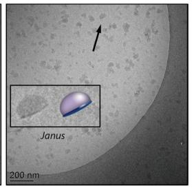
Fig. 5 The cryo-TEM images of hybrid particles obtained by the copolymerization of MMA: BA 90:10, at 80 °C, in the presence of 2.2 mM of the macroRAFT agent P(AA<sub>16</sub>-co-BA<sub>16</sub>)-TTC (M6) and 5 g L<sup>-1</sup> of Laponite® at pH 7.5 (R6).
