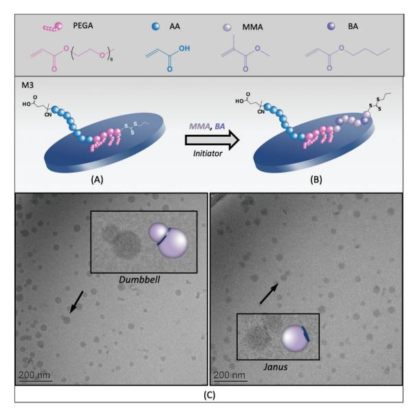
Fig. 2 Schematic representation of Laponite® platelets (A) with the adsorbed macroRAFT agent PAA<sub>40</sub>-b-PPEGA<sub>4</sub>-TTC (M3) and (B) during the synthesis of P(MMA-co-BA)/Laponite® nanocomposite latexes by RAFT-mediated surfactant-free emulsion polymerization using M3. (C) The cryo-TEM images of hybrid particles obtained by the copolymerization of MMA: BA 80:20, at 80 °C, in the presence of 2.2 mM of the macroRAFT agent M3 and 5 g  $L^{-1}$  of Laponite® at pH 7.5 (R3B).
