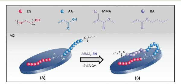
Fig. 1 Schematic representation of Laponite® platelets (A) with the adsorbed macroRAFT agent PEG<sub>45</sub>-b-PAA<sub>42</sub>-TTC (M2) and (B) during the synthesis of P(MMA-co-BA)/Laponite® nanocomposite latexes by RAFT-mediated surfactant-free emulsion polymerization using M2.
