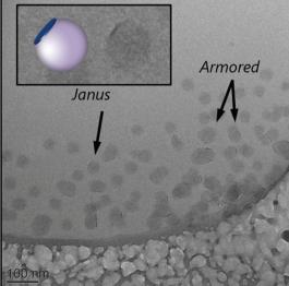
Fig. 4 The cryo-TEM images of hybrid particles obtained by the copolymerization of MMA: BA 90:10, at 80 °C, in the presence of 2.2 mM of the macroRAFT agent P(PEGA<sub>5</sub>-co-BA<sub>3</sub>)-TTC (M5) and 5 g L<sup>-1</sup> of Laponite® at pH 10 (R5B).
