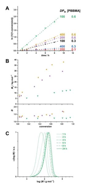
**Fig. 1** RAFT solution polymerization of **PBBMA** in DMAc at 70 °C. (A) First-order kinetic plots for various [**PBBMA**] and DP<sub>th</sub>. Dashed lines correspond to linear fits. (B) Evolution of number-average molar mass (top) and dispersity (bottom) with **PBBMA** conversion for [**PBBMA**] = 0.6 M at various DP<sub>th</sub>. (C) Size-exclusion chromatograms of polymers obtained at different times for [**PBBMA**] = 0.6 M and DP<sub>th</sub> = 100.
