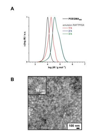
Fig. 2 (A) Size-exclusion chromatograms of polymers obtained by PBBMA emulsion RAFTPISA in water/ethanol 3:1 vol/vol at 70 °C with POEGMA<sub>500</sub> at DP<sub>th</sub> = 100, and 20 wt% solids content (entry 4 from Table S2†). (B) Transmission electron micrograph of nanoparticles obtained in the conditions mentioned above, after 2 h.
