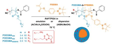
Scheme 1 Synthetic route and compounds employed in the current study for boron-rich nanoparticle formation by RAFT polymerization-induced self-assembly (RAFTPISA). ACVA = 4,4'-azobis(4-cyanopentanoic acid). AIBN = azobisisobutyronitrile.
