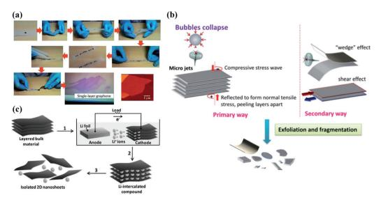
Fig. 6 Schematic diagram of top-down methods. (a) Flow chart of mechanical exfoliation method based on scotch tape. Reproduced with permission.<sup>97</sup> Copyright 2015, The Royal Society of Chemistry. (b) Illustration of the liquid phase ultrasonic exfoliation method. Reproduced with permission. 97 Copyright 2015, The Royal Society of Chemistry. (c) Schematic diagram of the intercalation assisted exfoliation method. Reproduced with permission. 98 Copyright 2011, Wiley-VCH.
