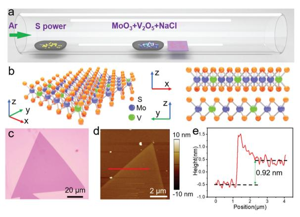
Fig. 1 (a) Schematic of synthesis of V-doped MoS<sub>2</sub> by CVD. (b) Atom structure and side view of V-doped MoS<sub>2</sub>. (c) Optical image of a V-doped MoS<sub>2</sub> single crystal. (d and e) AFM topography and thickness measurement of V-doped MoS<sub>2</sub>.
