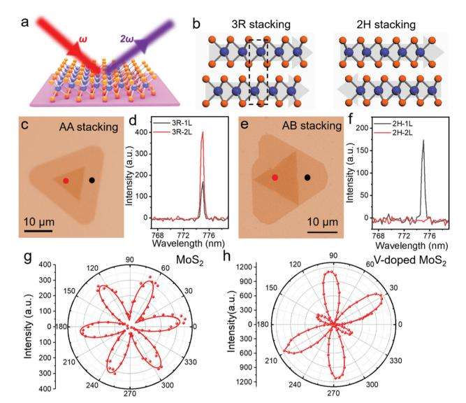
Fig. 4 (a) Schematic diagram of SHG process. (b) Side view of bilayer 3R and 2H phase  $MoS_2$  with different stacking order. (c and e) Optical images of  $MoS_2$  with 3R and 2H stacking. (d and f) Layer number-dependent SHG response 3R and 2H phase V-doped  $MoS_2$ . (g and h) Angular-dependent SHG intensity of monolayer  $MoS_2$  and V-doped  $MoS_2$ .
