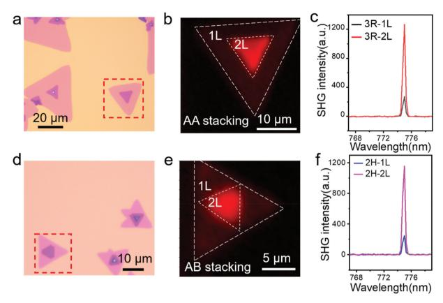
Fig. 5 SHG mapping of bilayer 3R and 2H phase V-doped MoS<sub>2</sub>. (a and d) Optical images of V-doped MoS<sub>2</sub> with 3R and 2H stacking. (b and e) SHG intensity mapping of V-doped MoS<sub>2</sub> flakes from (a and d), marked by red dashed boxes. (c and f) Layer number-dependent SHG response 3R and 2H phase V-doped MoS<sub>2</sub>.
