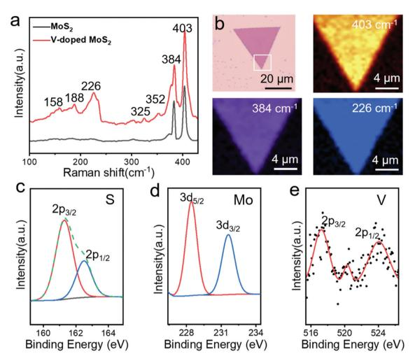
Fig. 2 Raman and XPS measurement of V-doped MoS<sub>2</sub>. (a)Raman spectra of pristine MoS<sub>2</sub> and V-doped MoS<sub>2</sub>. (b) Optical image of V-doped MoS<sub>2</sub> and its corresponding Raman intensity mapping images at 403 cm<sup>-1</sup>, 384 cm<sup>-1</sup> and 226 cm<sup>-1</sup>. (c-e) XPS narrow spectra of the S 2p, Mo 3d, and V 2p orbitals, respectively.
