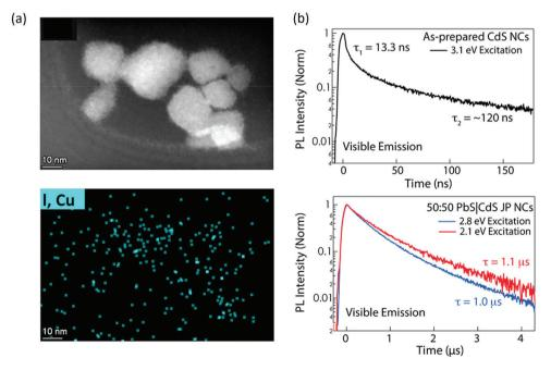
Fig. 5 (a) STEM image and EDS image area for Cu doped CsPbBr<sub>3</sub> nanocrystal photocatalysts. The figure was adapted from ref. 57 with permission from American Chemical Society. (b) Decay dynamics of photogenerated charge carriers in CdS nanocrystals and CdS/PbS Janus nanocrystals. Elongate charge separation of ~1 µs is observed with Janus structure. The figure was adapted from ref. 80 with permission from American Chemical Society.
