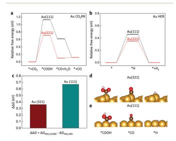
Fig. 5 Free energy diagrams for (a) CO<sub>2</sub>RR producing CO and (b) HER on Au(111) (black) and Au(321) (red). (c) Relative reaction free energy  $(\Delta\Delta G)$  for CO<sub>2</sub>RR compared to HER for Au(111) and Au(321). Optimized adsorption structures on (d) Au(321) and (e) Au(111) are presented. Asterisk (\*) indicates adsorbed species on the surface. The yellow, brown, red, and pink balls indicate Au, C, O, and H atoms, respectively.
