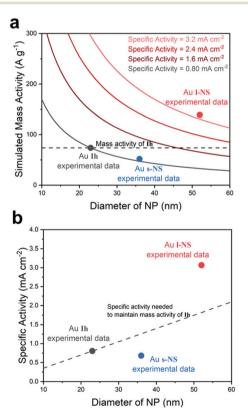
Fig. 3 (a) The relation between the NP diameter and simulated mass activity. Solid lines indicate specific activities one, two, three, and four times larger than that of Ih (0.80 mA cm $^{-2}$ ) at -0.7 V (vs. RHE). The dashed line is a trade-off line for retaining the mass activity of Ih. (b) The relation between the NP diameter and specific activity. The dashed line indicates the specific activity needed to maintain the mass activity of Ih.
