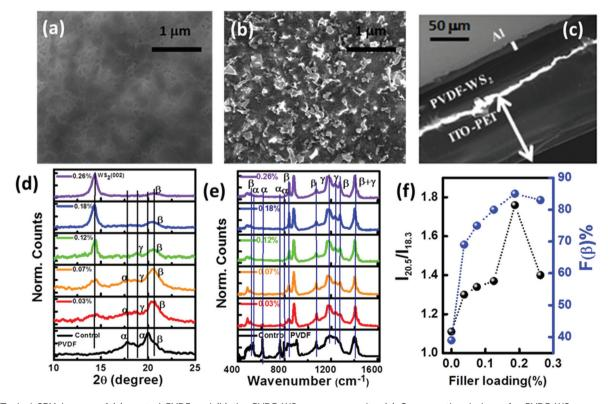
Fig. 1 Typical SEM images of (a) control PVDF and (b) the PVDF-WS2 nanocomposite. (c) Cross-sectional view of a PVDF-WS2 nanogenerator device. (d) X-ray diffraction patterns and (e) Fourier transform infrared spectra of control PVDF and PVDF-WS2 nanocomposite films at various WS2 filler loadings, (f) variation of intensity ratio  $\frac{I_{20.5}}{I_{18.3}}$  from the XRD pattern and relative  $\beta$ -phase content from FTIR spectra as a function of the WS<sub>2</sub> filler content.
