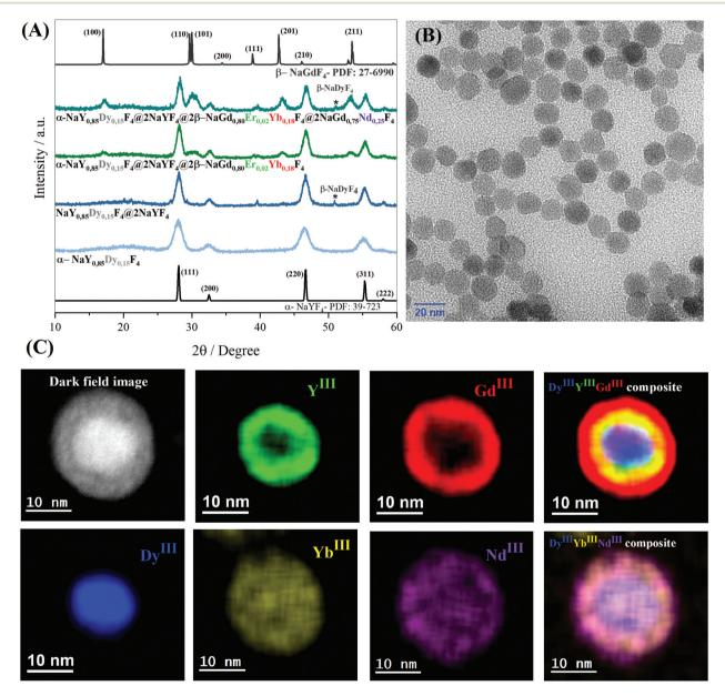
Fig. 2 (A) P-XRD data compared with references: α-NaYF<sub>4</sub> (PDF no. 77-2042) and β-NaYF<sub>4</sub> (PDF no. 16-334. (B) Bright field TEM image. (C) EDS  $elemental\ mapping\ of\ the\ \alpha-NaY_{0.85}Dy_{0.15}F_4@\alpha-NaYF_4@\beta-NaGd_{0.80}Er_{0.02}Yb_{0.18}F_4@\beta-NaGd_{0.75}Nd_{0.25}F_4\ nanoparticle.$
