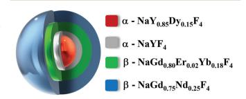
Fig. 1 Schematic illustration of the core@multi-shell nanoarchitecture.
