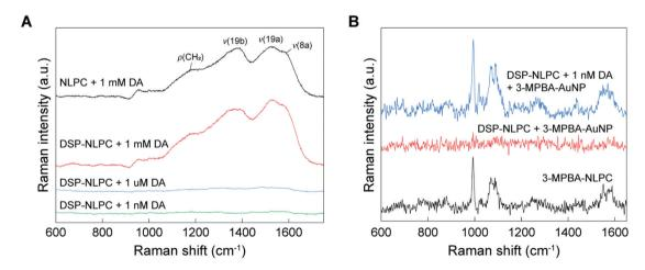
Fig. 4 3D NLPC-based DA detection using label-free and Raman tag-labeled SERS sensing. (A) Raman spectra for DA on the NLPC substrates functionalized with and without DSP for label-free SERS sensing at different DA concentrations. (B) Raman spectrum for the DA-specific dual-recognition structure at 1 nM DA, compared with configurations without DA and/or Raman tag-conjugated AuNPs.
