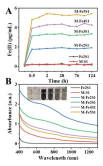
Fig. 2 Optimizing FeS NP biosynthesis. (A) Fe(II) produced from the reduction of Fe(III)-citrate by *S. oneidensis* MR-1. (B) UV-vis-NIR absorption spectra of *S. oneidensis*-FeS NPs. Fe2-Fe5 refers to different Fe(III)-citrate dosages from 2 to 5 mM. S1 refers to 1 mM thiosulfate. M refers to *S. oneidensis* MR-1. Control groups include S1 + Fe2 (without cells) and M + S1 (without Fe(III)-citrate).
