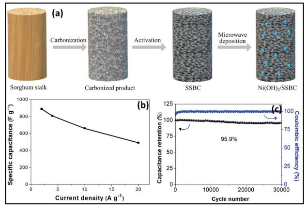
Fig. 18 (a) Synthesis of  $Ni(OH)_2$ /sorghum stalk biomass carbon, (b) specific capacitance of  $Ni(OH)_2$ /sorghum stalk biomass carbon composite and (c) cyclic property and columbic efficiency of  $Ni(OH)_2$ /sorghum stalk biomass carbon composite. Reprinted (adapted) with permission from ref. 267, copyright (2020), Elsevier B.V. All rights reserved.
