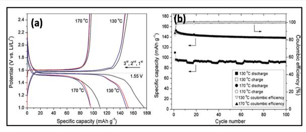
Fig. 21 (a) Galvanostatic charge/discharge curves for  $Li_4Ti_5O_{12}$  prepared at 130 °C and 170 °C between 1 and 2.5 V at a current density of 200 mA  $g^{-1}$ . (b) Cycling performance of  $Li_4Ti_5O_{12}$  prepared at 130 °C and 170 °C measured at a current density of 200 mA  $g^{-1}$ . Reprinted (adapted) with permission from ref. 281, copyright (2012), Elsevier B.V. All rights reserved.
