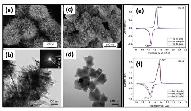
Fig. 20 (a and c) SEM images of  $\text{Li}_4\text{Ti}_5\text{O}_{12}$  synthesized at 130 °C and (b and d) TEM images of  $\text{Li}_4\text{Ti}_5\text{O}_{12}$  synthesized at 170 °C. (e and f) CV curves of  $\text{Li}_4\text{Ti}_5\text{O}_{12}$  prepared at (e) 130 °C and (f) 170 °C in the first three cycles at a scan rate of 0.2 mV s<sup>-1</sup>. Reprinted (adapted) with permission from ref. 281, copyright (2012), Elsevier B.V. All rights reserved.
