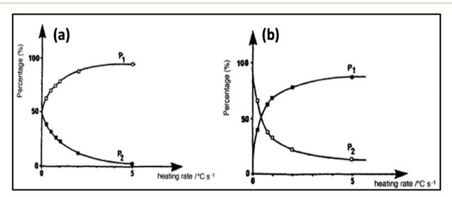
Fig. 5 Controlling rate of reaction using MW heating: (a) induced heating and (b) inversion heating. (113 Reprinted (adapted) with permission from ref. 113, copyright (1993), Elsevier B.V. All rights reserved.
