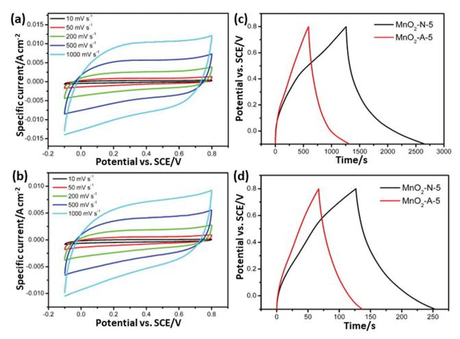
Fig. 16 (a and b) CV curves of MnO<sub>2</sub>-N-5 and MnO<sub>2</sub>-A-5 at different scan rates and (c and d) charge/discharge curves of MnO<sub>2</sub>-N-5 and MnO<sub>2</sub>-A-5 at current densities of 0.2 A g<sup>-1</sup> and 1 A g<sup>-1</sup>, respectively.<sup>257</sup> Reprinted (adapted) with permission from ref. 257, copyright (2013), Elsevier B.V. All rights reserved.
