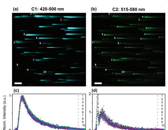
Fig. 6 Equal temporal behavior of several agglomerates of  $UC_{Tm}@Rh110$ . NIR-LSM images of the same region of  $UC_{Tm}@Rh110$  sample under 975 nm excitation ( $F_d = 0.9 \text{ J cm}^{-2}$ ) in (a) channel 1 (C1: 420–500 nm; 560 V) and (b) channel 2 (C2: 515–580 nm; 635 V). Time-resolved normalized intensity profiles of numbered agglomerates in (c) channel 1 and (d) channel 2. Scale bar: 50  $\mu$ m.
