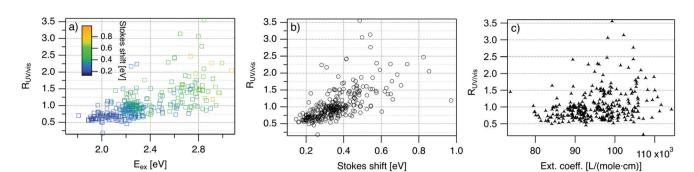
Fig. 4  $R_{\text{UV/Vis}}$ , ratio of areas of UV excitation peak (Region 2) to excitation peak (Region 1), as a function of (a)  $E_{\text{ex}}$ , (b) SS, and (c) extinction coefficient of the template DNA strand, calculated using the nearest neighbor model. <sup>64,65</sup>
