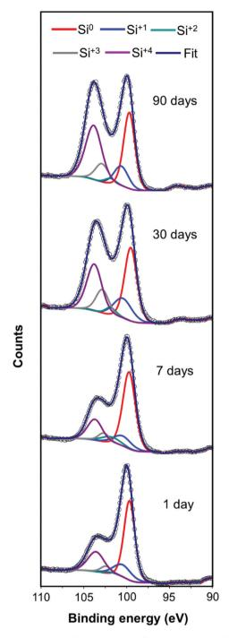
Fig. 5 High resolution XP spectra of the Si 2p region of mp-Si300 NPs at different times after the synthesis and storage under ambient conditions. For clarity, only  $2p_{3/2}$  peaks of different oxidation states are shown.
