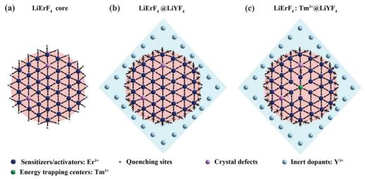
Fig. 3 (a) The energy migration quenching processes in a LiErF<sub>4</sub> UCNP. (b) A typical strategy to reduce the energy migration to surface quenching sites through an inert-shell coating. (c) The approach of simultaneously preventing energy migration quenching processes through introducing Tm<sup>3+</sup> ions as energy trapping centers.
