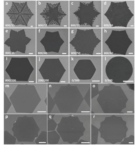
Fig. 5 SEM images of GFs grown on a liquid Cu surface with different shapes formed by varying the Ar:  $H_2$  ratio (a–l). Reprinted with permission from Springer Nature, NPG Asia Materials<sup>74</sup> (self-organized graphene crystal patterns, B. Wu *et al.*, 2013). Formation of tips in hexagonal graphene grains by incremental additions to the CH<sub>4</sub> flow (m–r). Reprinted with permission from ref. 75. Copyright 2014 Wiley-VCHd. All scale bars are 5 μm.
