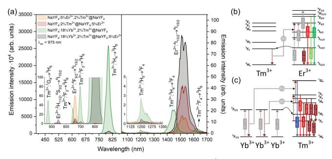
Fig. 5 (a) Emission of core@shell NPs under excitation by 975 nm laser radiation (15 W cm<sup>-2</sup>). Left spectra were measured with a CCD camera, whereas right spectra used a NIR PMT. (b and c) Mechanisms responsible for the observed emission in UCNPs doped with (b) Er<sup>3+</sup> and Tm<sup>3+</sup> or (c) Yb<sup>3+</sup> and Tm<sup>3+</sup> lanthanide ions under 975 nm laser excitation.
