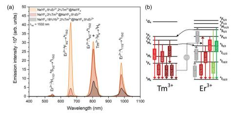
Fig. 7 (a) Emission of synthesised core@shell NPs under 1532 nm laser excitation (15 W cm $^{-2}$ ). (b) Possible energy transfers in NPs doped with Er $^{3+}$ and Tm3+ ions under 1532 nm laser excitation.
