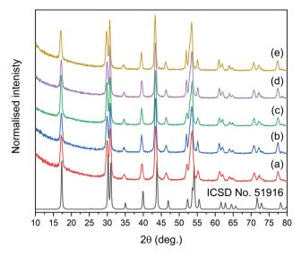
Fig. 1 XRD patterns of synthesised core@shell NPs: (a) NaYF<sub>4</sub>:2% Tm³+@NaYF<sub>4</sub>, (b) NaYF<sub>4</sub>:2%Tm³+,5%Er³+@NaYF<sub>4</sub>, (c) NaYF<sub>4</sub>:2% Tm³+@NaYF<sub>4</sub>:5%Er³+, (d) NaYF<sub>4</sub>:18%Yb³+,2%Tm³+@NaYF<sub>4</sub>, and (e) NaYF<sub>4</sub>:18%Yb³+,2%Tm³+@NaYF<sub>4</sub>. The ICSD reference represents the XRD pattern of  $\beta$ -NaYF<sub>4</sub> with a hexagonal structure.
