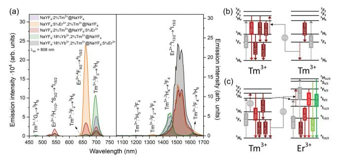
Fig. 4 (a) Emission of core@shell NPs in the Vis and NIR range under excitation by 808 nm laser radiation (15 W cm<sup>-2</sup>). On the left, spectra were measured using a CCD camera, whereas spectra on the right used an NIR PMT (b and c) possible energy transfer schemes in NPs doped with (b) Tm<sup>3+</sup>or (c) Er<sup>3+</sup> and Tm<sup>3+</sup> ions under 808 nm laser excitation.
