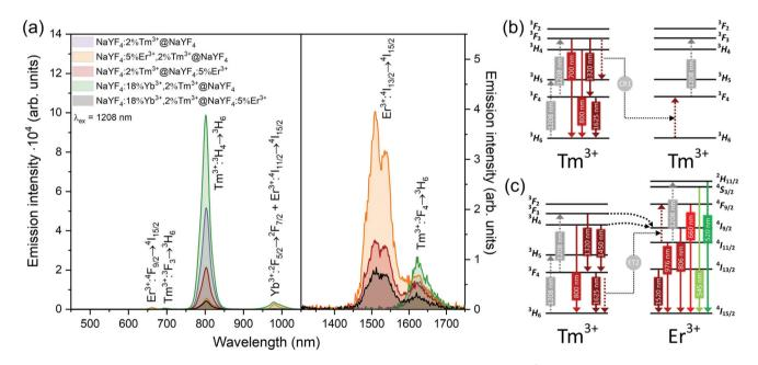
Fig. 6 (a) Emission of core@shell NPs collected under excitation by 1208 nm laser radiation (15 W cm<sup>-2</sup>). Left spectra were measured using a CCD camera and right spectra used a NIR PMT. (b and c) Simplified UC mechanisms responsible for the observed emission of NPs doped with (b) Tm<sup>3+</sup> or (c) Er3+ and Tm3+ ions under 1208 nm laser excitation.
