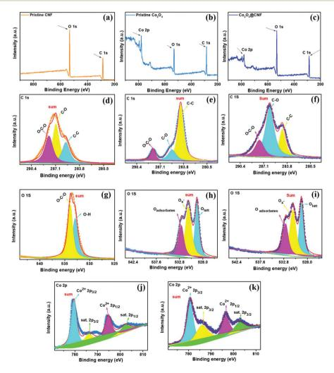
Fig. 3 (a-c) XPS survey spectra of pristine CNF, pristine Co<sub>3</sub>O<sub>4</sub> nanoparticles and 1D Co<sub>3</sub>O<sub>4</sub>@CNF hybrid; (d-f) C 1s binding energy region, (q-i) O 1s binding energy region and (j and k) Co 2p binding energy region for the respective samples.
