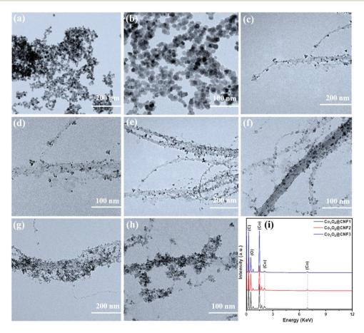
Fig. 1 TEM images at higher and lower magnification (a and b) of pristine Co<sub>3</sub>O<sub>4</sub> nanoparticles, (c and d) 1D Co<sub>3</sub>O<sub>4</sub>@CNF1, (e and f) 1D Co<sub>3</sub>O<sub>4</sub>@CNF2 and (q and h) 1D Co<sub>3</sub>O<sub>4</sub>@CNF3 hybrid nanostructure. (i) The elemental spectra of the 1D Co<sub>3</sub>O<sub>4</sub>@CNF1, 1D Co<sub>3</sub>O<sub>4</sub>@CNF2 and 1D Co<sub>3</sub>O<sub>4</sub>@CNF3 hybrid nanostructure.
