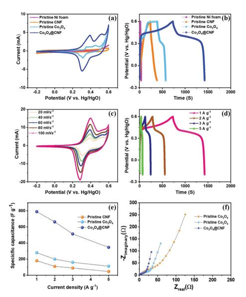
Fig. 5 Comparison of three electrode electrochemical measurements for the pristine Co<sub>3</sub>O<sub>4</sub> nanoparticles, pristine CNF and 1D Co<sub>3</sub>O<sub>4</sub>@CNF: (a) CV curve at 20 mV s<sup>-1</sup> of scan rate, (b) GCD curve of 1 A q<sup>-1</sup> of current density, (c and d) CV and GCD curves at various scan rates and current densities, (e) specific capacitance and (f) EIS measurement.
