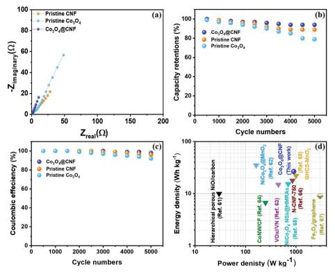
Fig. 7 Electrochemical performance of the SSC devices for the pristine Co<sub>3</sub>O<sub>4</sub> nanoparticles, pristine CNF and 1D Co<sub>3</sub>O<sub>4</sub>@CNF hybrid electrodes: (a) EIS plot, (b and c) capacity of retentions and coulombic efficiency of electrodes at 15 A g<sup>-1</sup> of current density over 5000 cycles and (d) Ragone
