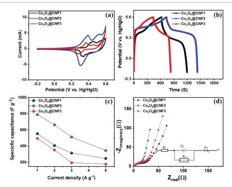
Fig. 4 Electrochemical performance of the three-electrode measurement for the 1D Co<sub>3</sub>O<sub>4</sub>@CNFx hybrid electrodes (where x means the feeding amount of the Co<sub>3</sub>O<sub>4</sub> nanoparticles on the CNF surface): (a) CV curve at 20 mV s<sup>-1</sup> of scan rate, (b) GCD curve of 1 A g<sup>-1</sup> of current density, (c) specific capacitance at the various current densities and (d) electrochemical impedance spectra (EIS).
