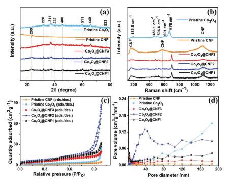
Fig. 2 (a) XRD pattern, (b) Raman spectra, (c and d) adsorption-desorption isotherm and BJH curves of the CNF, Co<sub>7</sub>O<sub>4</sub> nanoparticles, 1D Co<sub>3</sub>O<sub>4</sub>@CNF3, 1D Co<sub>3</sub>O<sub>4</sub>@CNF2 and 1D Co<sub>3</sub>O<sub>4</sub>@CNF1 hybrids.
